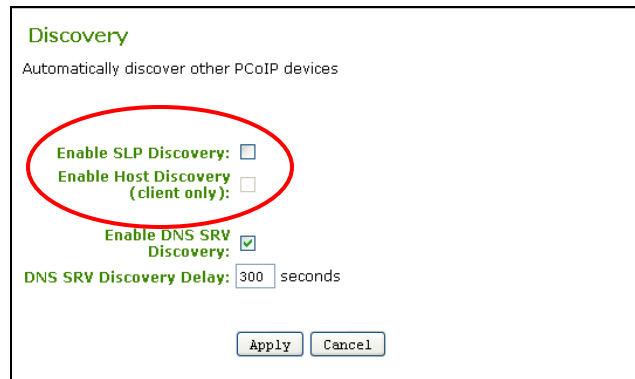
Figure 7: Disabling SLP and Host Discovery under Configuration → Discovery in the zero client web interface.
