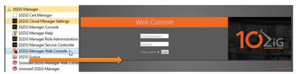
The Web Console will open up in your default selected browser. Note, if the Cloud Connector is installed locally, this port will be used by default for accessing the Web Console. Enter in your user name if using a local account or domain and username for a domain account.
