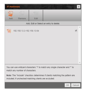
Lastly, ensure that the filter with the new filer rules is enabled by checking box next to the filter name.
