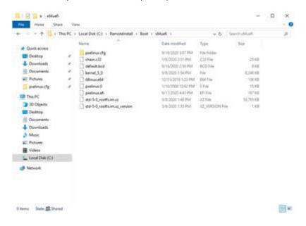
3. In the ..\Boot\x64uefi\pxelinux.cfg path, we need to delete the default file and rename the recovery.cfg to default.
