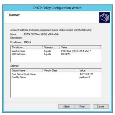
20. Lastly, verify that the policies for the scope have been activated. If not activated, rightclick on the Policies and select Activate. The policies should take effect and properly dish out the correct options with the appropriate filtering.
